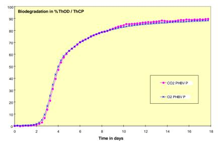
**Fig. 2:** PHBV powder degradation, aqueous system,  $20^{\circ}$ C. Standardized presentation of O<sub>2</sub>-consumption and CO<sub>2</sub> -production by Theoretical Oxygen Demand, (ThOD) and Theoretical Carbon- dioxide Production (ThCP)
