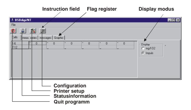
figure 1: display structure of BSBdigi
