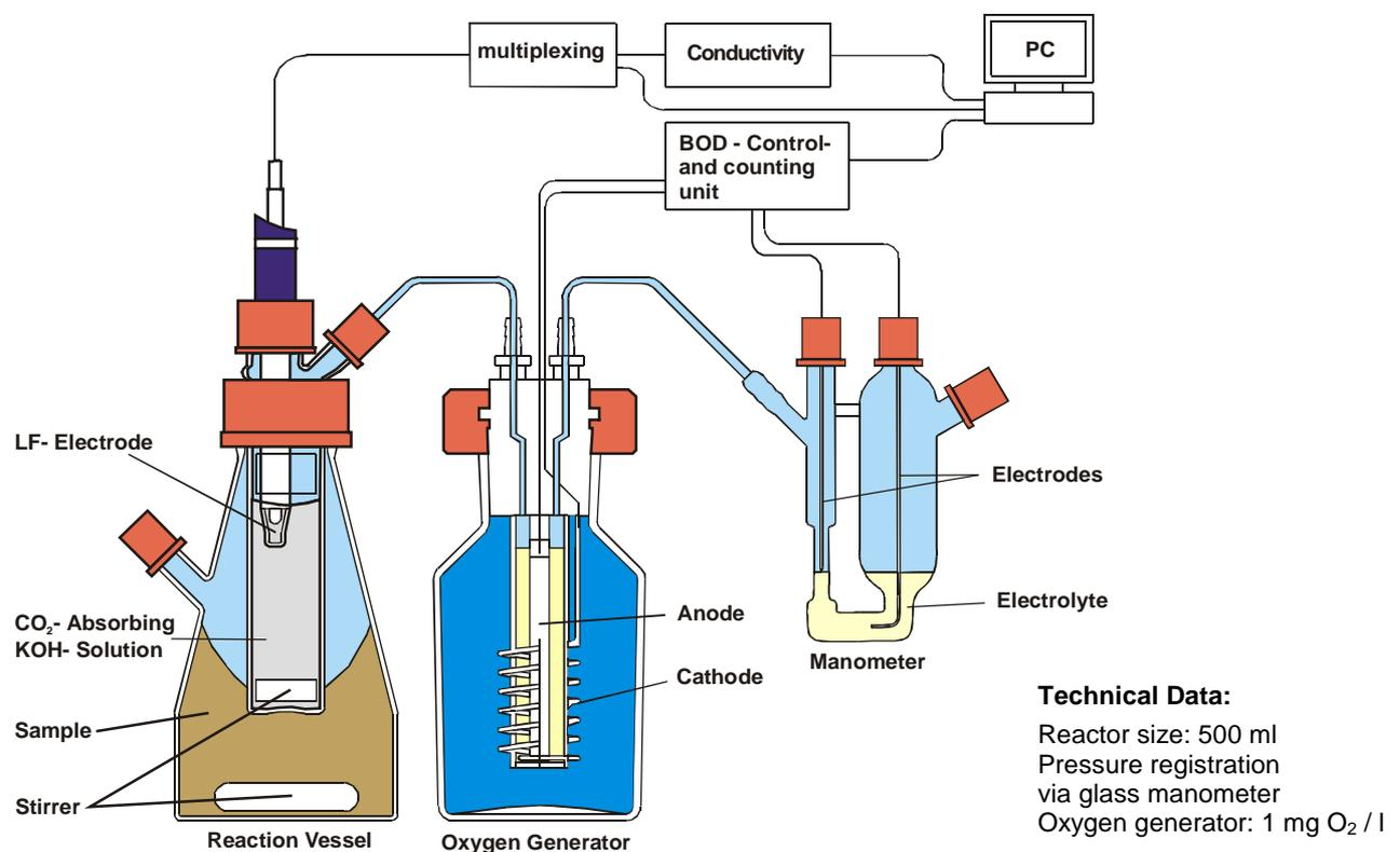
**Fig. 1** Improved closed-circuit respirometer at constant pressure, with both, continuous restoration of O<sub>2</sub> consumed and detection of CO<sub>2</sub> produced
