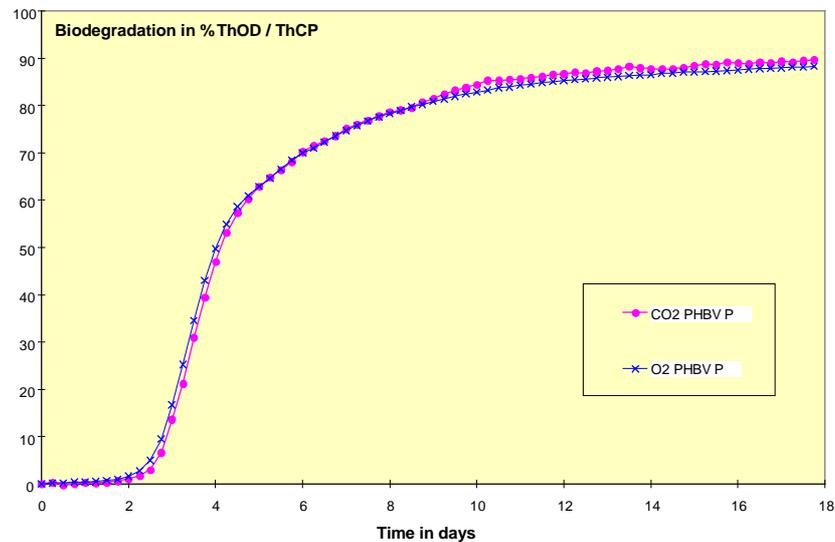
**Fig. 2:** PHBV powder degradation, aqueous system, 20°C. Standardized presentation of O<sub>2</sub>-consumption and CO<sub>2</sub> -production by Theoretical Oxygen Demand, (ThOD) and Theoretical Carbon-dioxide Production (ThCP)
